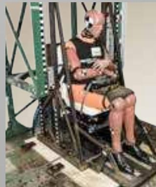
The picture on the left shows the SideRiser 2 set up with a test dummy with a mass of 30 stone. The agreed test was to drop the seat from ever
